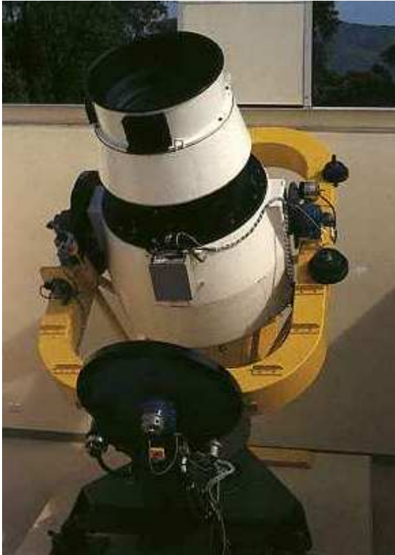
Figure 7.1: The Automated Patrol Telescope. Figure 7.2: A sample APT image of NGC 6633.
