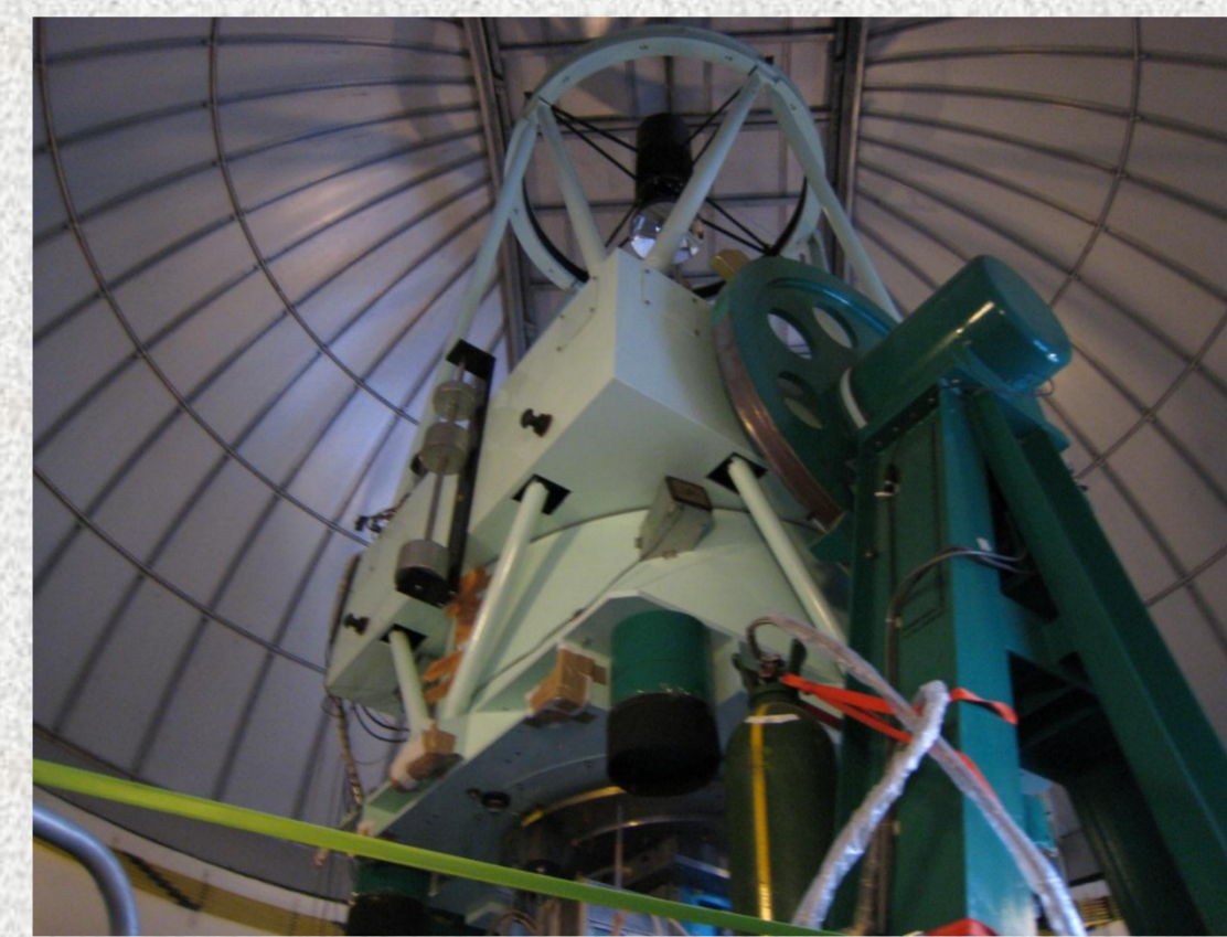
Fig.3: IRSF telescope. SIRIUS is installed at the Cassegrain focus. (Photo by Takuya Suenaga)
